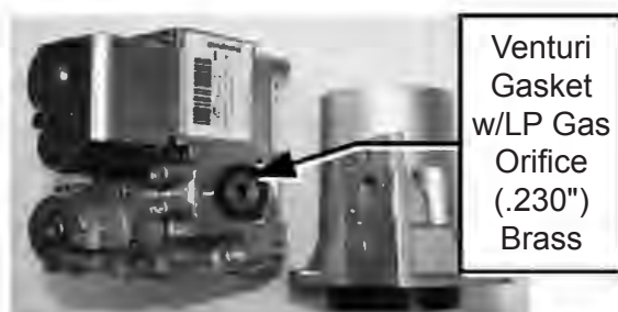
Gas Control with .230" Propane (LP) Orifice
