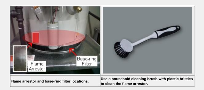
If there are no flammable vapors or liquids near the water heater, check the base-ring filter (around the base of the unit) and flame arrestor (underneath the base of the unit) for dust or dirt. If the base-ring filter is dirty, clean it using a vacuum cleaner with a brush attachment. If the flame arrestor is dirty, clean it using a household cleaning brush with plastic bristles. Next, check to make sure that the vent system isn't blocked and that the water heater is getting enough air.
