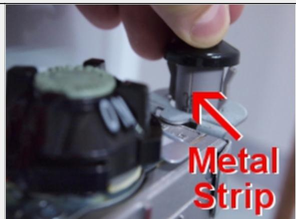
On vertically mounted igniters, the metal strip should face left toward the gas valve housing.
