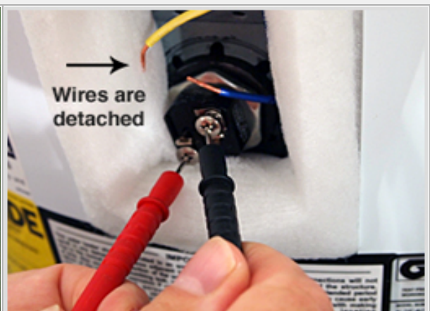
Use a multimeter to measure the resistance of the upper heating element. A good element will have a resistance of between 5-25 Ohms.
